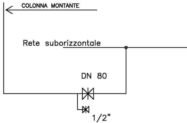
SCHEMA ATTACCO AUTOPOMPA V.V.F. RETE GENERALE
