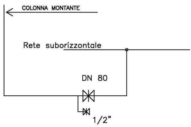
SCHEMA ATTACCO AUTOPOMPA V.V.F. RETE GENERALE
